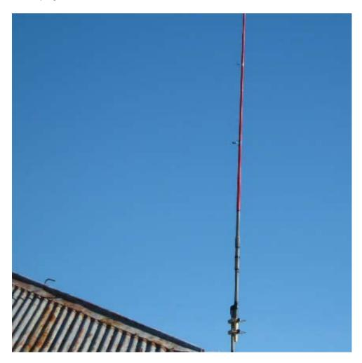
I started at the top of the rod by putting the wire through the ferrule and tying it to the swivel. I then close wound the wire down to the butt of the rod. In doing this I added extra wire (different coloured wire) to take it down to the butt. Total length of wire is 100 metres plus. The joining of the wires, I twisted them and then I used coax seal.
